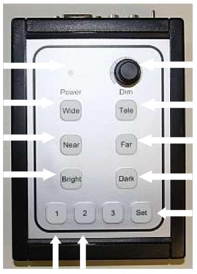
The buttons 1 and 2 are memory buttons, 2 different camera settings can be stored and recalled.
