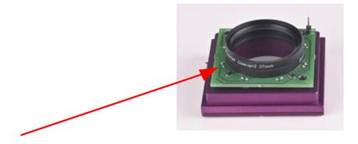
Now you can adjust the distance by using the various close up lenses. Please chose the close up lenses according the table above The reassembly occurs in reverse order.
