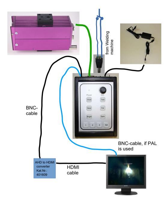
When using an AHD monitor, e.g. our No. 401367, the AHD/HDMI converter and the HDMI cable are not required
