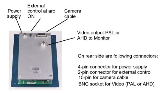
A close contact (free of potential in Ext. Control), e.g., from a welding machine, enables automatic switching from memory 1 to memory 2 which saves normally camera parameters during welding, i.e. zoom, sharpness and brightness.
