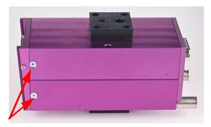
Remove this screws, also on opposite side Remove the front plate with the LED ring light For reassembling please check the polarity of the connector
